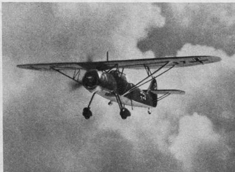
German Henschel-126 is larger and faster than our own Air O. P.'s, resembles our discarded O-46. Unlike U. S. types, the Hs-126 has high parasol wing and is armed with three to five 7.9-mm. machine guns.
